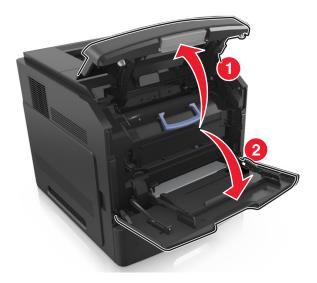
**2** Lift the blue handle, and then pull the toner cartridge out of the printer.
